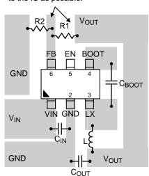
LX should be connected to inductor by wide and short trace, and keep sensitive components away from this trace.
