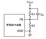
Figure 1. Cff Capacitor Setting
