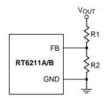
Figure 5. Output Voltage Setting
