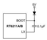
Figure 6. External Bootstrap Diode
