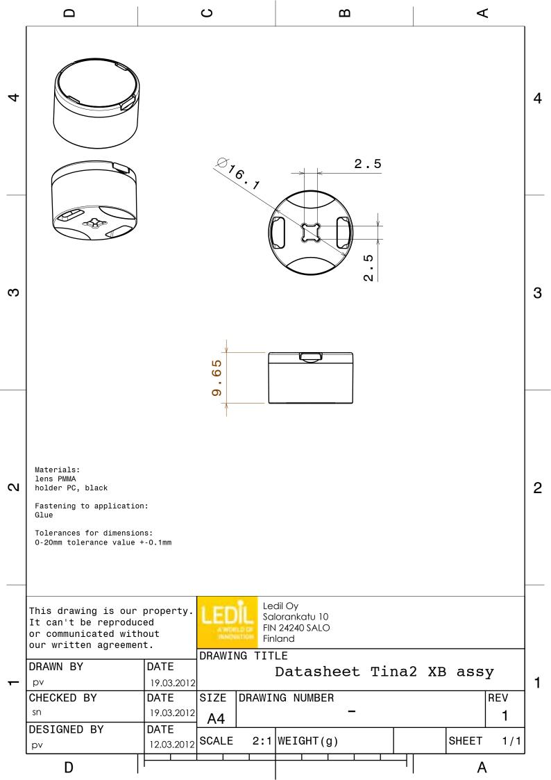
Luminaire: LEDIL OY CP12672\_TINA2-M (XB-D) Efficiency=82% Lamps: 1 x Cree XB-D white (97Im @ 250mA)
