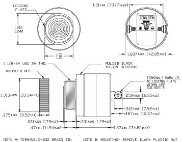
NOTE A: TERMINALS-.032 BRASS TIN PLATED, TAPPED FOR #6-32 SCREW. TWO #6-32 NICKEL PLATED BRASS SCREWS INCLUDED. WILL ACCEPT 1/4' QUICK CONNECT. NOTE B: MOUNTING- REMOVE BLACK PLASTIC NUT AND INSERT THREADED FRONT THROUGH 1.25' HOLE PUNCHED IN PANEL, IF DRIENTATION IS NEEDED, NOTE LOCKING FLATS ON DRAVING. SCREW NUT BACK ON. DO NOT OVERTIGHTEN.
