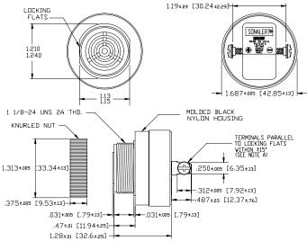
NOTE A: TERMINALS-.032 BRASS TIN PLATED, TAPPED FOR #6-32 SCREW. TWO #6-32 NICKEL PLATED BRASS SCREWS INCLUDED. WILL ACCEPT 1/4' QUICK CONNECT. NOTE B: MOUNTING- REMOVE BLACK PLASTIC NUT AND INSERT THREADED FRONT THROUGH 1.25' HOLE PUNCHED IN PANEL, IF DRIENTATION IS NEEDED, NOTE LOCKING FLATS ON DRAWING. SCREW NUT BACK ON. DO NOT OVERTIGHTEN.
