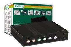
For transmitted RGB signals over CAT 5 cable with more than 150 meter the skew delay becomes significant and a correction is necessary. Below 150 meter the delay is negligible. This unit allows a perfect skew delay correction of the video signals for a brilliant and sharp picture.
