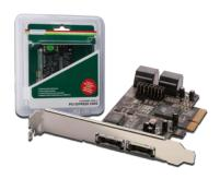
4 x internal Serial ATA connectors, 2 x external eSATA connectors (selectable)
