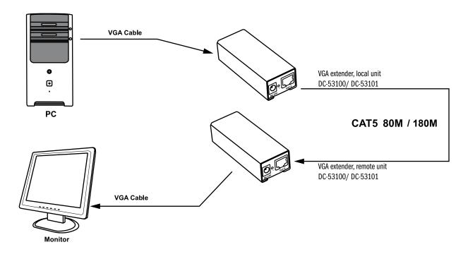
Examples of use 2 - Cat5 VGA extender/splitter and Cat5 VGA video selector:
